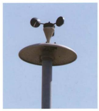
The ISC Infinity 2000 perimeter detection system utilizes a "WX-75M" weather station. This fully integrated monitoring sub-system detects environmental changes resulting from wind and precipitation and supplies the necessary data to the system processor. Based on this continuously updated flow of information the processor constantly adjusts sensor operating parameters to eliminate the generation of environmentally induced false alarms.
